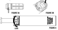
Rotate the lock ring to locked position following the arrow in Figure 6 until it can no longer be rotated. The lock ring should rotate approximately 180°. Audible clicks will be heard during this process.
